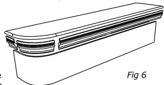
Next offer up the riser moulding to determine where the tread will sit. Trim the tread sections to width and the rear section to depth. The rear tread section will usually also need to be trimmed to fit around the newel post. Finally trim the straight riser moulding sections to length and your bull nose step is ready to install.
