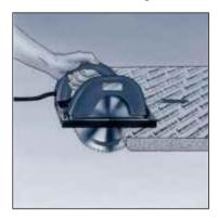
When using an electric saw you should start from the decorative profiled front edge cutting the Worktop face down.
