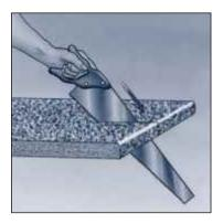
When using a handsaw the decorative face should be uppermost and again you should start from the decorative profiled front edge keeping the saw at a low angle to ensure the best cut. Ensure that your saw is sharp and well set and has 10/12 teeth per inch.
